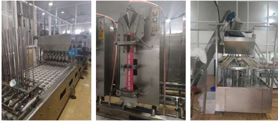
Gambar 27. Mesin Filling : (a) Cup , (b) Pack , dan(c) Botol
